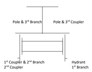
In the above diagram the runners have been positioned on the reel to run to the right hand plug. If running to the left hand plug the hydrant runner will change to the left hand side of the reel and the hoses and first coupling will be set up in the tray to run to the left hand side.
